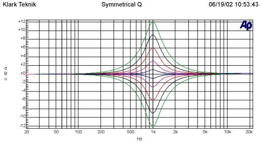
This class of equaliser has the same curves in boost as the constant-Q type, but then has cut responses that are symmetrical with the boost ones. In other words, the bandwidth in cut is defined not according to our usual definition of Q (see constant-Q above) but as "the point were the signal is cut by 3dB less than the maximum cut". Most equalisers described by their manufacturers as "Constant Q" in fact produce symmetrical responses.
